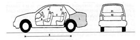
93cm/36" min. Α Cushion not compressed. В 96cm/37" min. Seat fully rearwards. C 61cm/41" min. Front seat fully rearwards. D 84cm/33" min. Cushion not compressed. Wheelbase Ε 245cm/96" min. F1 133cm/52" min. Interior width between doors 122cm/48" F2 Between armrests G 25cm/10" Point of measurement parallel with squab
